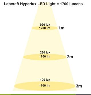
**LUX** levels are determined using a lux metre and is the measurement of the exact intensity of light at a given point away from the light unit. The Lux level will be influenced by the distance from the light source but also by a wide range of different factors including the product design, secondary lensing and the environment the light is fitted within.
