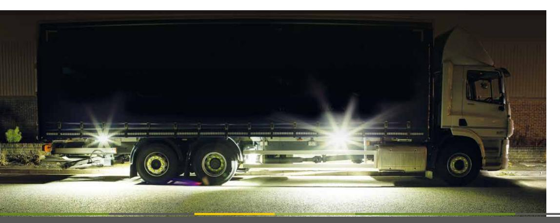
The Banksman is a manoeuvring aid that delivers additional bright white light to the sides of any vehicle where traditional reversing lights cannot cover.
